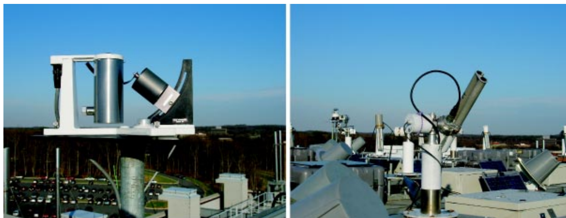
Fig. 1 UV-MFRSR shadowband radiometer, part of USDA UVMRP (left), and CIMEL sun/sky photometer, part of NASA AERONET network (right) were continuously run side by side at NASA GSFC in Greenbelt, Maryland (lat=39.03 deg N, long=76.88 deg W), in 2002 to 2004. The elevated location (the height of elevated platform at the roof of the building is ~20 m above ground and ~90 m above sea level) enables unobscured view of horizon by both instruments.
