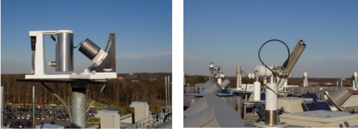
Figure 1. UV-MFRSR instrument (left) and CIMEL sun/sky photometer (right) were run side by side at NASA Goddard Space Flight Center in Greenbelt, Maryland in 2002-2003. The height of elevated platform at the roof of the building is ~20m above ground (~100m above sea level).
