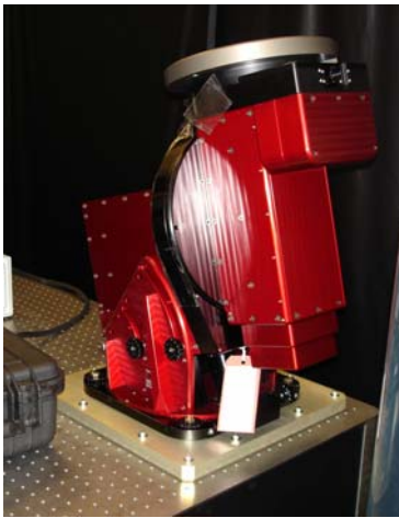
Figure 18 Solar tracker capable of supporting 150 pounds
