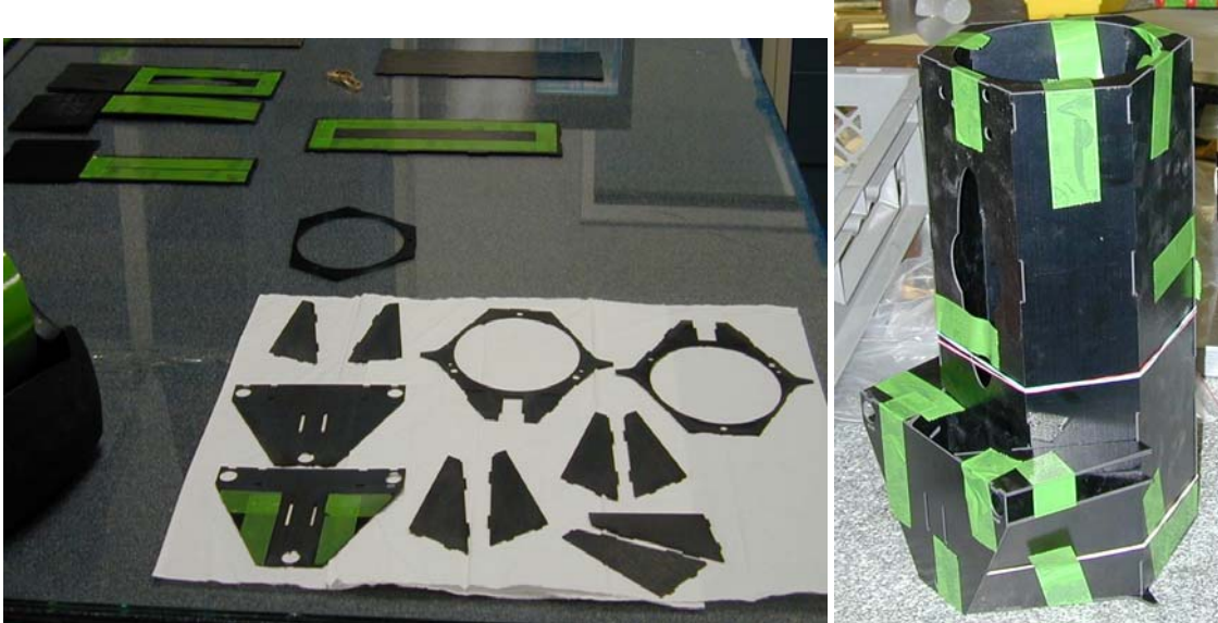
Figure 21 Pre-assembly parts for the hex-tube (left) and the assembled tube (right)
