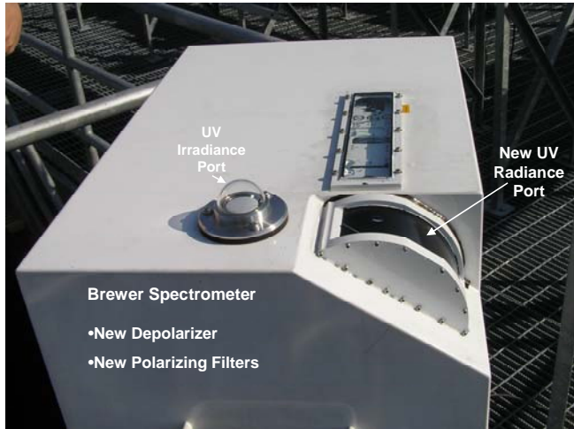
Figure 1: A photograph of the modified Mark III double Brewer spectrometer showing the curved radiance entrance port on the lower right.
