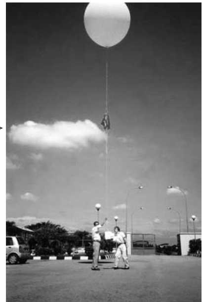
Malaysian Meteorological Service staff preparing an ozonesonde on the day of launch.
