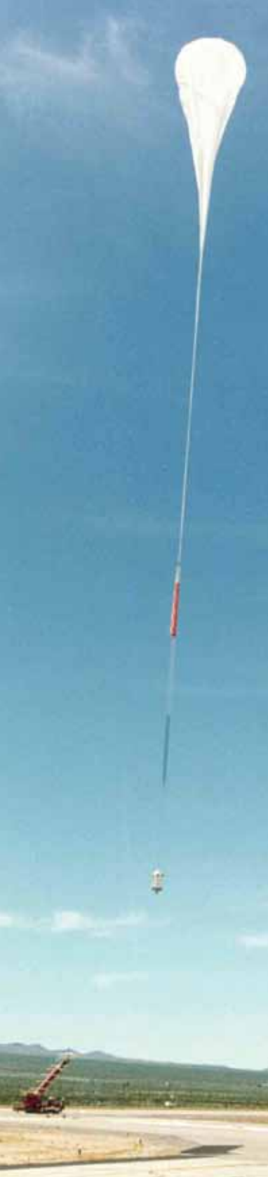
High altitude balloons can carry large payloads with complex instruments deep into the stratosphere. These balloons are launched using special equipment only once or twice a year.
