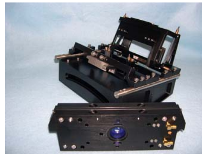
Brassboard camera with dual photoelastic modulator assembly in the foreground. (This multi-angle UV/V/NIR polarimetric spectrometer has been developed through ESTO IIP.)
