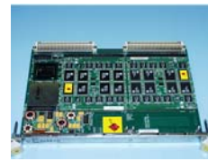
FPGA real-time processor board
