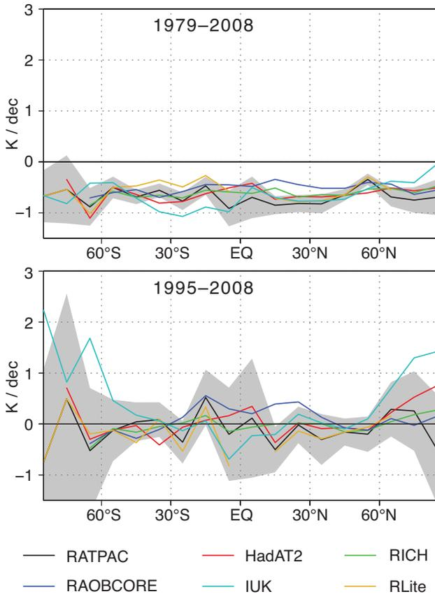
**Figure 4-6.** Zonal-mean temperature trends (K/decade) at 50 hPa from six adjusted radiosonde data sets for the periods 1979–2008 (top) and 1995–2008 (bottom). Gray shading indicates the 2-sigma trend confidence interval from the RATPAC data set (others are comparable). Trends are computed from temperature anomaly time series, omitting data for two years after the El Chichón and Mt. Pinatubo volcanic eruptions.
