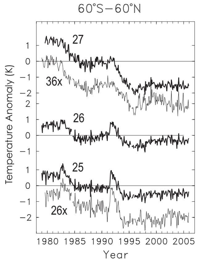
**Figure 4-8.** Time series of SSU temperature anomalies (K) for channels indicated (Figure 18 from Randel et al., 2009). Data for channels 26x and 36x are shifted for clarity. Exact weighting functions for the SSU satellite instrument can be found in Figure 1 of Randel et al. (2009). Channel 27 corresponds to ~34–52 km altitude, channel 36x to ~38–52 km, channel 26 to ~26–46 km, channel 25 to ~20–38 km, and channel 26x to ~21–39 km.
