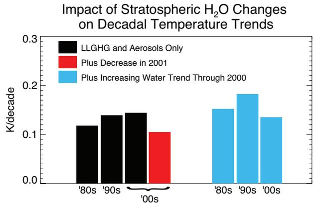
**Figure 4-18.** Decadal warming rates (K/decade) arising from (i) the long-lived greenhouse gases (LLGHG) and aerosols alone (black), as well as (ii) that obtained including the stratospheric water decline after 2000 (red) and (iii) including both the stratospheric water vapor decline after 2000 and the increase in the 1980s and 1990s (cyan). Based on Solomon et al. (2010).
