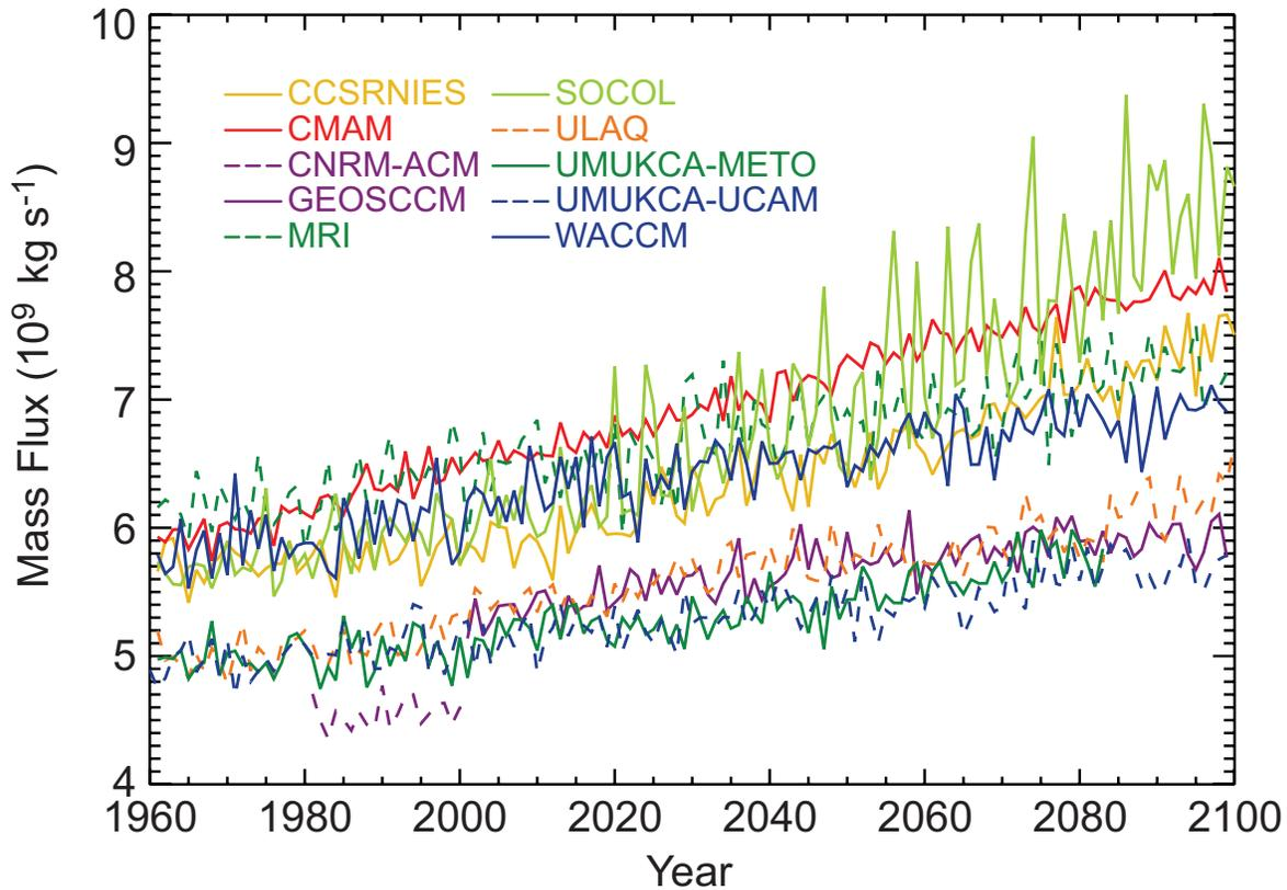
**Figure 4-16.** Annual mean upward mass flux ( $\text{kg s}^{-1}$ ) at 70 hPa, calculated from residual mean vertical velocity between the turnaround latitudes of the Brewer-Dobson circulation, for the simulations prepared for the CCM-Val SPARC report. See Table 3-1 in Chapter 3 of this Assessment for a description of the chemistry-climate models shown in the figure. Figure from Chapter 4 of SPARC CCMVal (2010).
